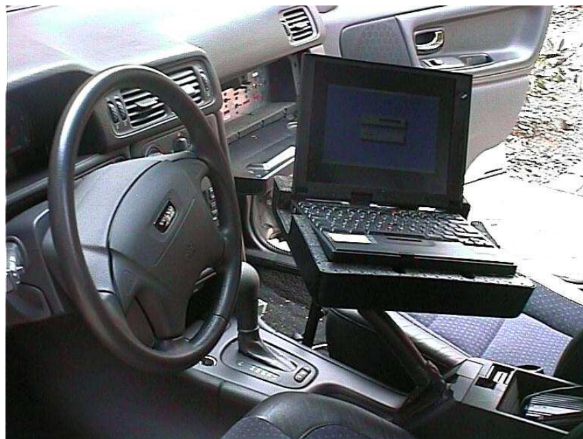
Figure 1 Notebook running the model-based diagnosis software on the Volvo demonstrator vehicle
